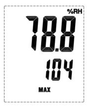
The upper reading is the real humidity value, the middle reading is the calibration value and the lower one is the MAX icon, which indicates the calibration value is above 75%RH. Press "▲" or "▼" button to increase or decrease the value, after finished calibration, press "HOLD" button to exit the Humidity Calibration Mode and the calibrated value will be kept automatically.
